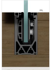
NOTE: Ensure adequate water drainage points! Not suitable for concrete slab concealing due to potential water retention
