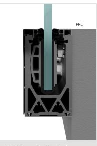
NOTE: When installing Versatilt as face mount, consider using our 1350mm high 'Clear glaze' glass to achieve height required for pool fencing
