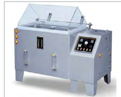
In-house salt spray testing - tests aluminium extrusion for durability of coating
